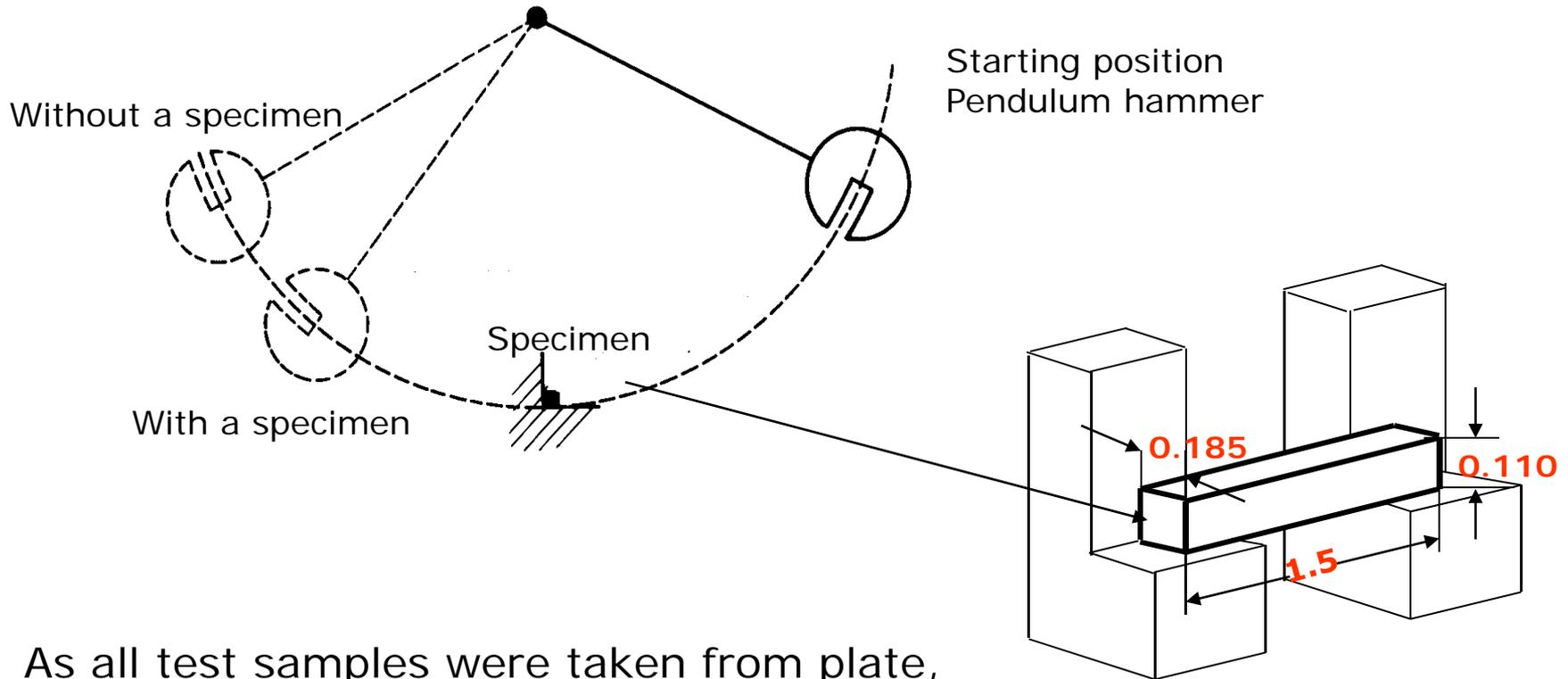
As all test samples were taken from plate, a tailor made unnotched impact sample was designed with dimension **0.110 x 0.185 x 1.5 inch** (non standard)
